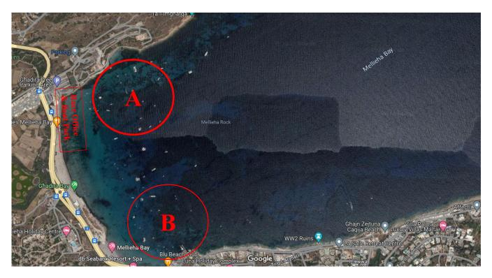
Coaches may tie their support vessels to one of the moorings located in areas A and B. When weather conditions are between 15-25+ knots coming from 30° to 75°, it is advisable to tie support vessel on a mooring located at area A.
