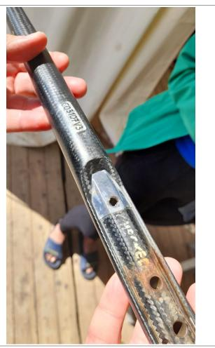
During a routine inspection of hull appendages, the equipment of BRA 137 was discovered to be carrying modification which is breaking class rule C.8.3(a). In more detail, the fuselage was carrying additional material which was not been registered by the manufacturer as in Class Rule B.1. See attached photo.
