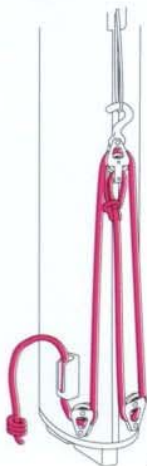
jib tension applied
